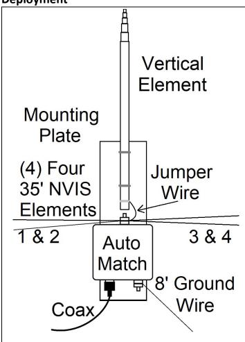
NOTE - Never loosen any permanently affixed bolts, washers, or nuts on the match.
