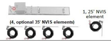
Step 6 - a) Attach the 1 o-ring connector of the Grounded Counterpoise element that has black shrink tube to the bottom bolt on the Alpha Match, as circled below. b) Secure the ring connector in place with the included nut.
