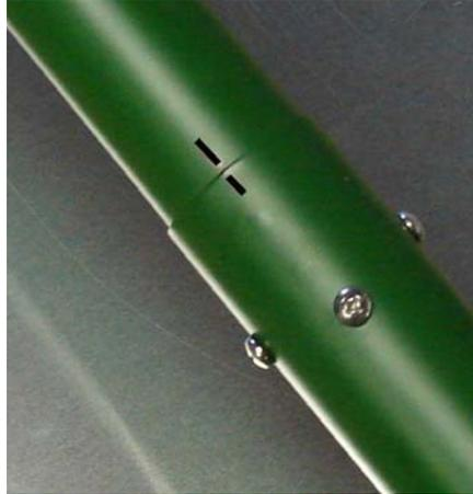
Continue with securing each section with their appropriate screws until all sections have been secured. Again, the bottom section has four screws, the middle sections have two screws and the top three sections have one screw.
