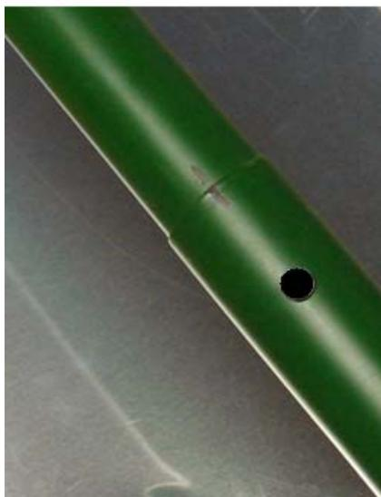
As mentioned, each tube section (except the top, tip section) requires screws for permanent base mounting to prevent the tubes from collapsing down into the larger diameter tubes immediately below it. Your antenna is now prepared to have the screws affixed, into each of the holes you have pre-drilled, as the following image of the base section shows.
