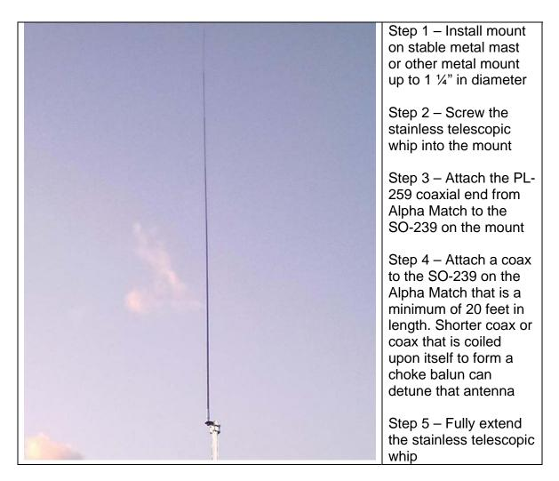
Tip – Radials/Counterpoise can help the performance of any vertical antenna system but are not required for the Alpha Antenna to function. If counterpoises are used, we recommend that four 25 foot 16, 14, or 12 gauge wires be affixed with ring connectors that can easily fit one per counterpoise under the washers on the supplied mount.
