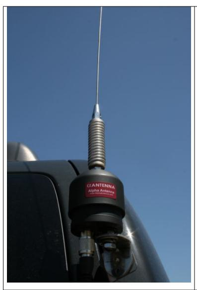
Step 1 – Install your mount to a stable metal part of your vehicle. We recommend our stainless steel Alpha Antenna Jam Mount.
