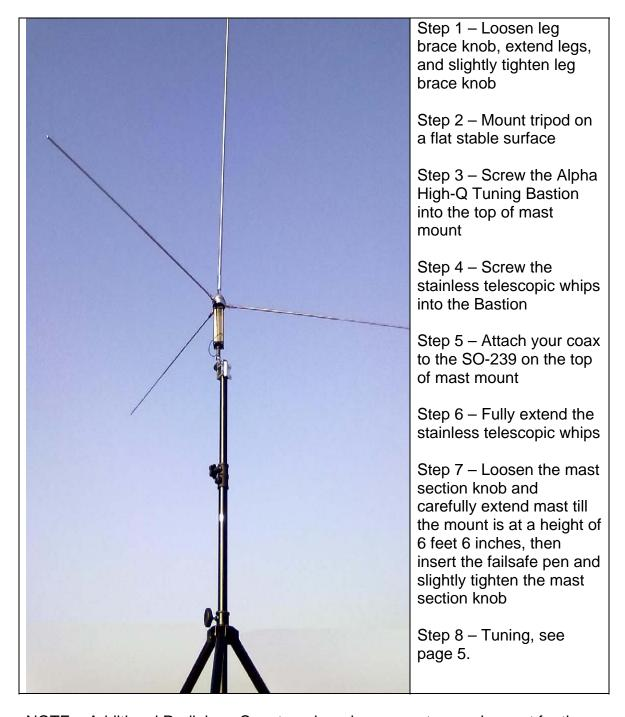
NOTE – Additional Radials or Counterpoise wires are not a requirement for the Alpha DX Antenna to function well, but when added can improve performance for frequencies below 7.3MHz. You must guy the antenna system with heavy nylon cord, high tensile string, or non-conductive material when winds are present.
