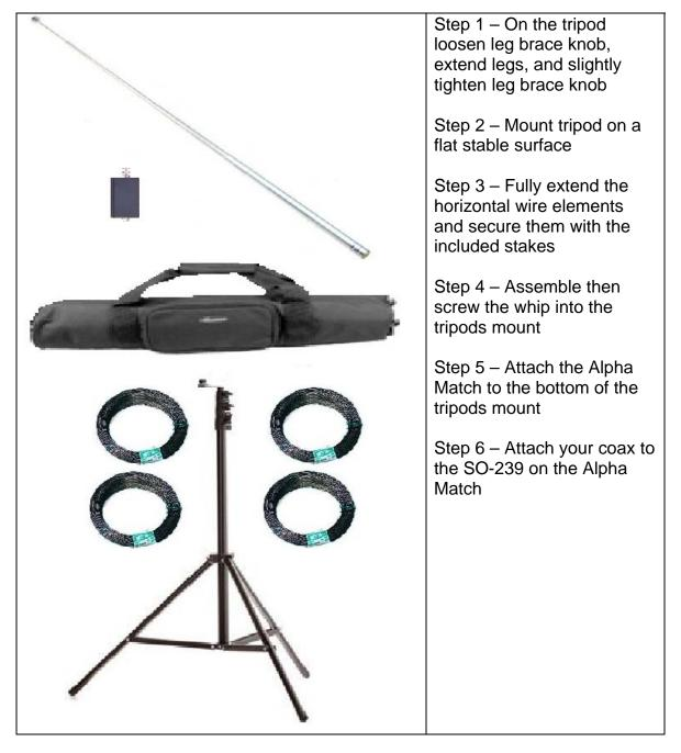
NOTE – Additional Radials or Counterpoise wires should not be used with the antenna system. All components of the antenna system are designed to exacting standards for high performance, including the tripod, which is designed to be your counterpoise system. We advise that you guy the antenna system with the included radiating elements.
