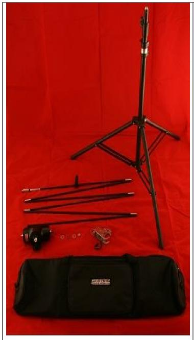
Step 1 – On the tripod loosen the leg brace knob, extend the legs, and slightly tighten the leg brace knob
