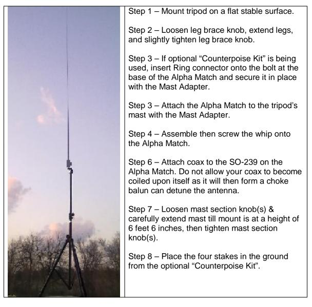
Tip – Counterpoise can help the performance of any vertical antenna but are not required for the Alpha Antenna to function. If they are used to enhance performance, then we recommend you use our Counterpoise Kit or your own wire run affixed with ring connectors affixed in the manner described above, utilizing four 15 foot or longer 16, 14, or 12 gauge wires
