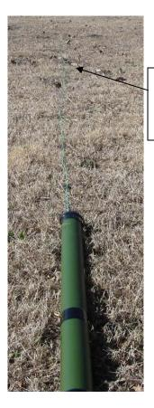
Pull wire straight out from base tube until it is fully extended along the ground
